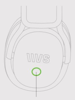
Hold power button for 3 seconds to power the headset on or off.
